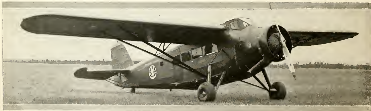
Latest type Pilgrim Model 100-A transport monoplane of American Airways equipped with Goodyear Air Wheels
